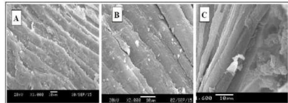
Fig.4.7 SEM images of composites containing (A) 20 %, (B) 25 % and (C) 35 % fibers of 35 mm length
