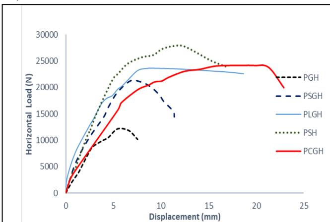
Fig.4 Horizontal load - displacement curve for tested pile specimens PSH, PGH, PSGH, PLGH and PCGH.
