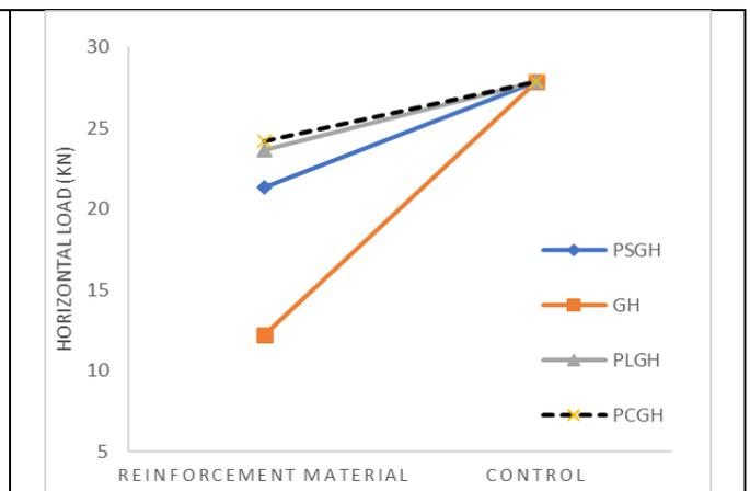
Fig.5 Horizontal load vs reinforcement material relationship for Horizontally loaded specimens
