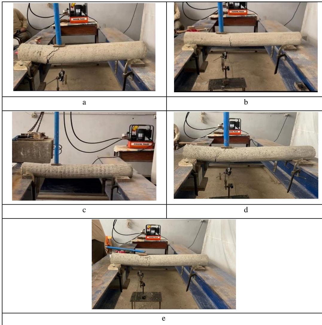
Fig.6 Modes of failure for horizontal loaded specimens
