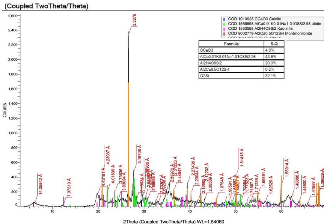
Fig. 6. X-ray diffraction patterns for the studied soils.
