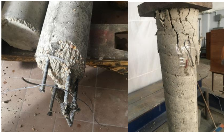
Fig.10: The failure of the failure of PCC piles.
