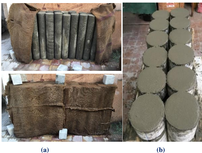
Fig.2: (a) curing conditions, (b) pile models.
