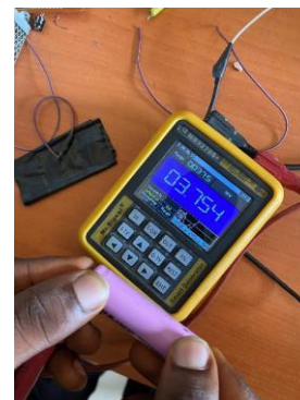
Fig. 5: Battery Test showing the Measured Voltage.
