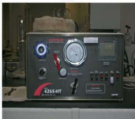
Fig.3.8 Ultrasonic Cement Analyzer
