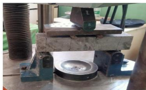
(A) Experimental setup for flexural strength test
