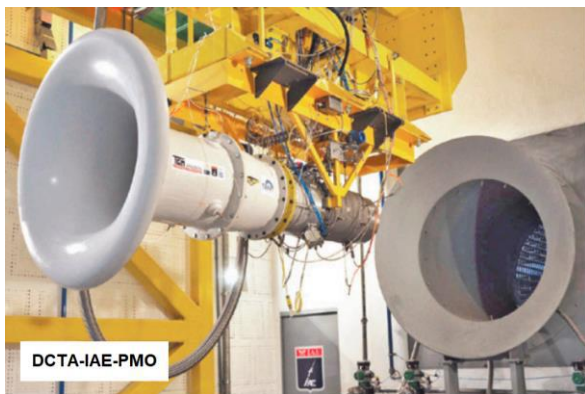
Fig. 1: Illustration of the aeronautic gas turbine investigated in this study on test rig.
