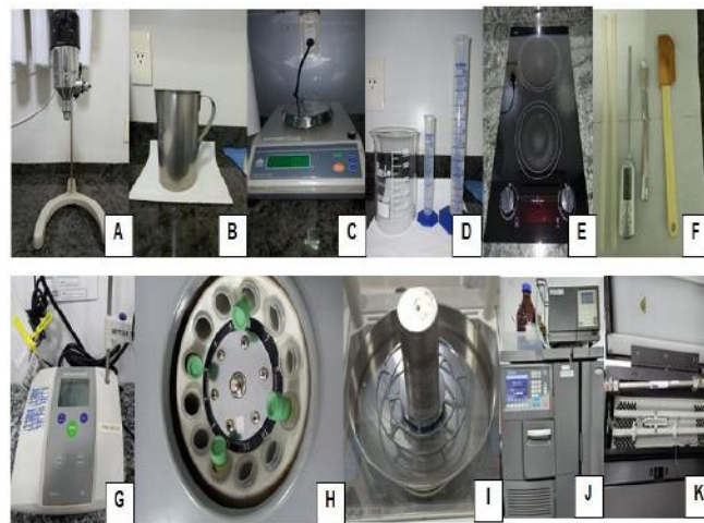
Fig.1. Equipment used for the physicochemical tests. A Fisatom model 713 mechanical stirrer; B stainless steel beaker; C Gehaka BG 4000 balance; D glassware; E hotplate; F plastic rod, digital thermometer, spatula and breadboard; G digital pH meter; H model 80-2 B centrifuge; I metal pycnometer; J HPLC; and K column.
