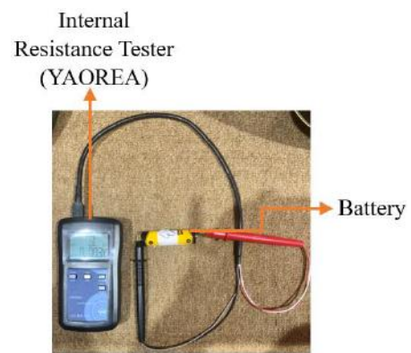
Fig. 3: Measuring battery internal resistance
