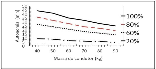
Fig.2 - Autonomy Versus Driver Mass
