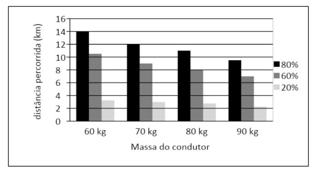
Fig.3 - Distance traveled versus conductor mass
