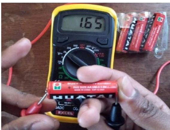
Fig. 28: Measurement of the electromotive force of a new AA battery.
