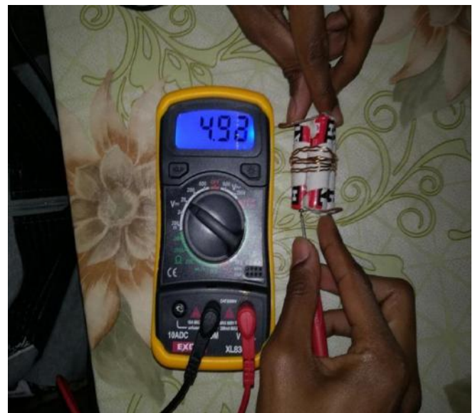
Fig. 30. Measurement of the electromotive force of three new batteries combined of size AA.
