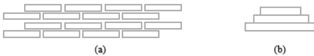
Fig. 3: Preventive measures against delamination using (a) staggered ply drops and (b) chamfered edges.
